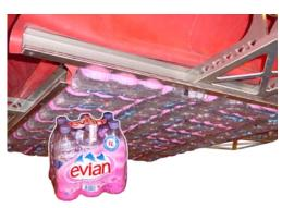
Whether it is one bottle, one row or an entire layer, palletizing or de-palletizing, thanks to the UniGripper solution, the BottleGripper offers the same possibilities as any other of his cousins in the UniGripper product range.
