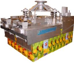
The main spare part for any UniGripper is the foam. Ease of maintenance is granted as the foam is glued on a foam carrier plate, which enables you to change the foam within matters of minutes.
