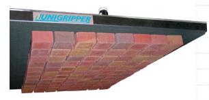
100% customized to each project, we build the UniGripper Customized to our well proven standard. The unique patented valve technology allows the Gripper to literally recognize if and where a product is located underneath it, and applies vacuum to the product only.
