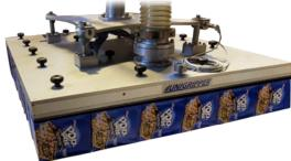
Almost all LayerGrippers are equipped with the floating attachment, and, depending on the products to handle, side clamps with or without side skirts.
