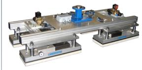
Even our Standard Module System turns out to be a fully customizable and capable vacuum gripper, both as a stand-alone unit or integrated into other more complex systems.
