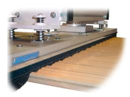
TimberGripper is also superior in handling materials, with milled out grooves or holes.
